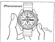
When depressing the fly-back button, the second hand slips from the 0 position.
